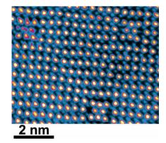
Novel self-assembled nanorods with a neodymium-rich core are discovered in neodymium and titanium codoped bismuth ferrite. The three-dimensional atomic structure and chemistry of these nanorods is determined using a combination of scanning transmission electron microscopy and density functional calculations. The theoretical studies show that these may function as one-dimensional semiconducting channels through the ceramic.
