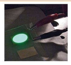
A new family of anthracene core emitters where the lowest triplet state has less than half the energy of the next highest triplet level is developed. The triplet fusion becomes highly efficient, resulting in fluorescent organic light emitting diode (OLED) devices of very simple structure, that far exceed the 25% external quantum efficiency limit due to the efficient singlet generation from triplet fusion in the device.
